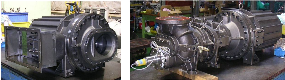
Fig. 2.1 Semi-hermetic motor and compressor. (left : motor, right ; built compressor and motor)
